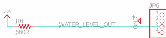
Figure 9: Water Level Sensor Schematic
